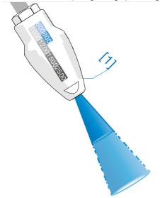
Rotor nozzle when opening the high-pressure gun
