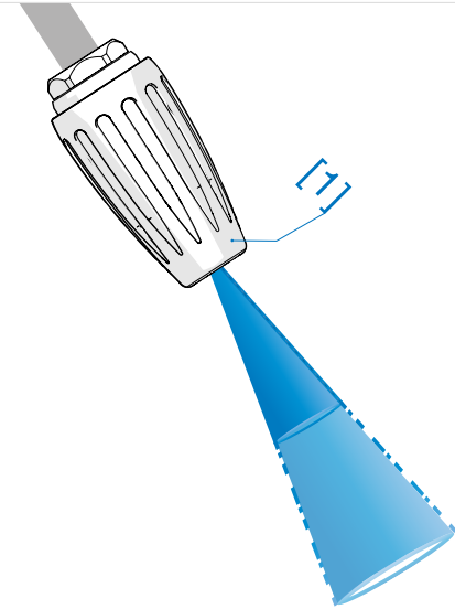
Rotor nozzle when opening the high-pressure gun
